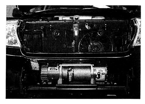
10. Fit the bracket and bolt to the original chassis
