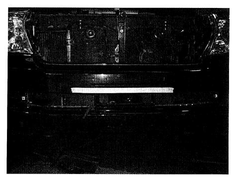
6. Cut the section under the number plate joining the upper and lower section of the bumper
